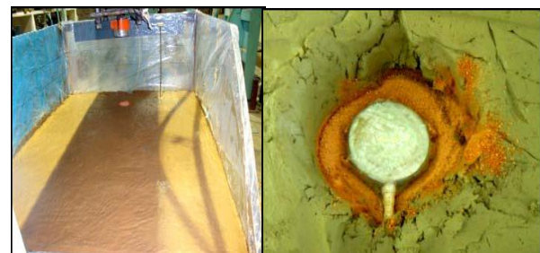
(c) Placing of earth pressure cells and settlement peg
