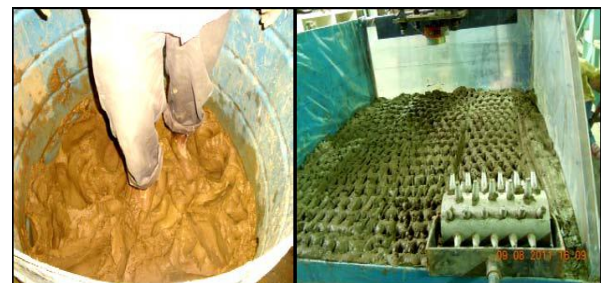
(b) Kneading compaction using sheep foot roller
